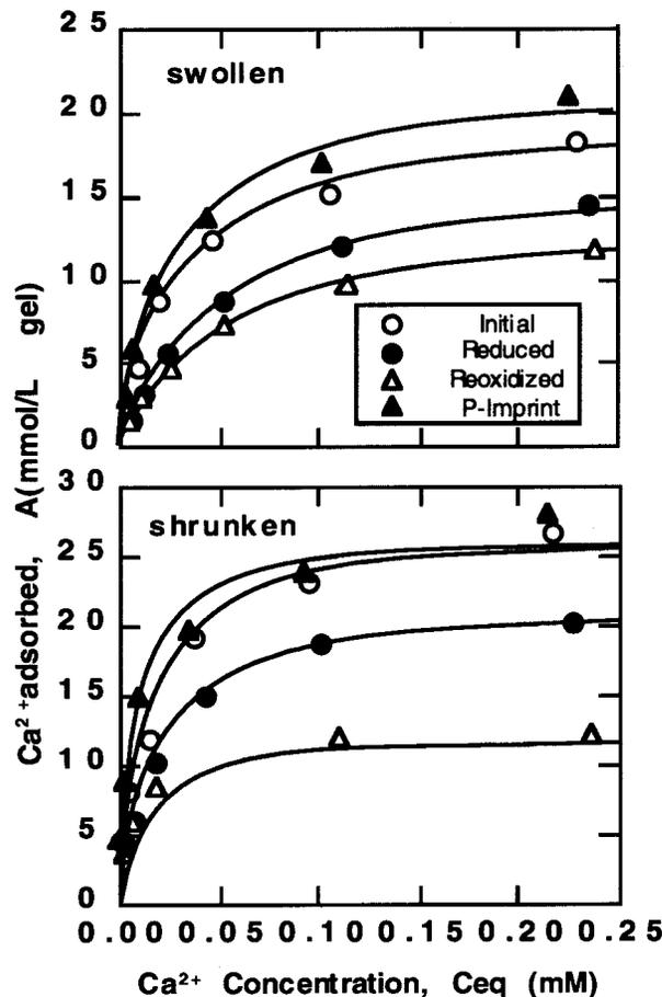
**Figure 2.** Adsorption of calcium ions by the various types of imprinted gels, each containing 40 mM BAC. The swollen state was measured at 25 °C and the shrunken state at 60 °C. In each case, the adsorption curves closely follow a Langmuir isotherm.
