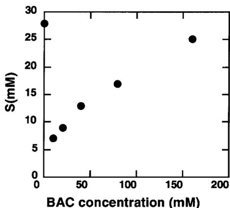
**Figure 3.** Saturated adsorption capacity,  $S$ , as a function of the BAC concentration in the reoxidized gels in the shrunken state.  $S$  increases with the BAC concentration. In the case of the gel having no BAC, there is no frustration in the  $\text{Ca}^{2+}$  adsorption, and  $S$  is higher than for the other cases.
