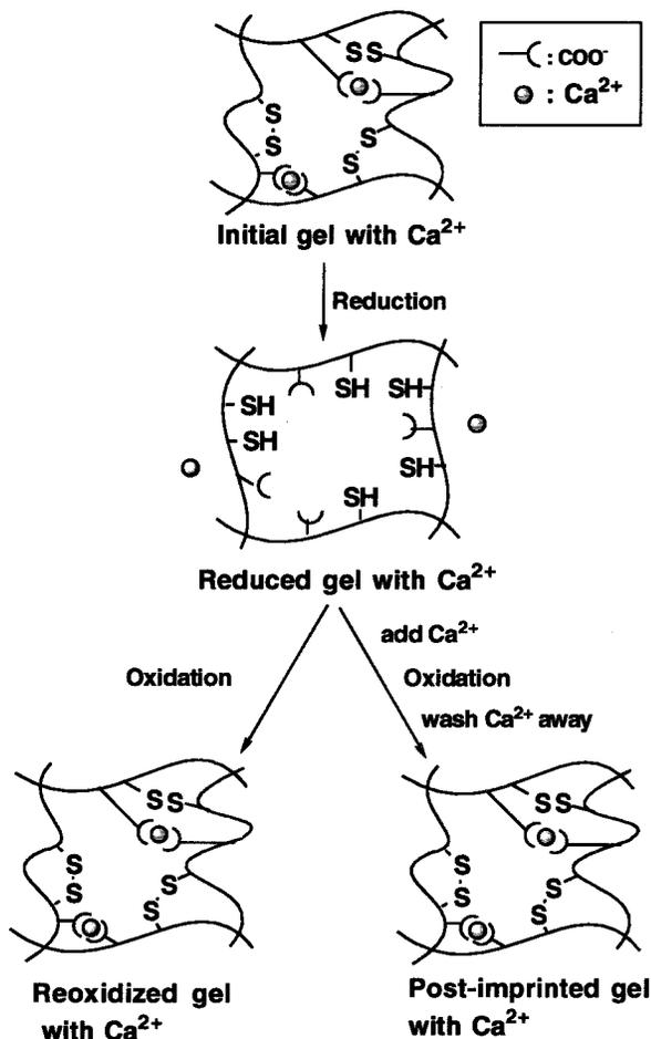
**Figure 1.** Schematic illustration of the procedure for preparing the modified imprinted gels, showing the expected S–S bond formation. The initial gels, reoxidized gels, and post-imprinted gels are expected to have the same conformation, even after re-formation of the S–S bonds. Calcium ions are present under the measurement conditions for the gels. The initial gels, reoxidized gels, and post-imprinted gels are expected to show the same calcium absorption affinity.
